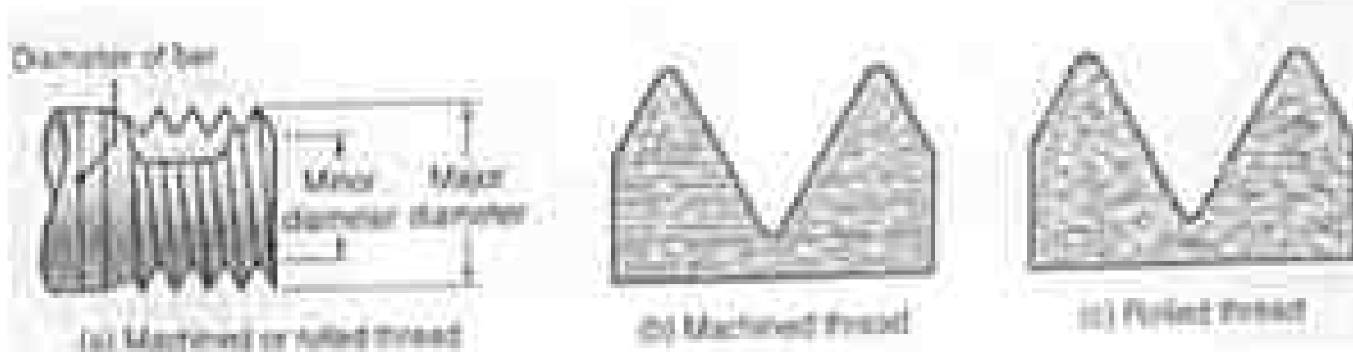
FIGURE 13.17 (a) Features of a machined or rolled thread. Grain flow in (b) machined and (c) rolled threads. Unlike machining, which cuts through the grains of the metal, the rolling of threads imparts improved strength because of cold working and favorable grain flow.
