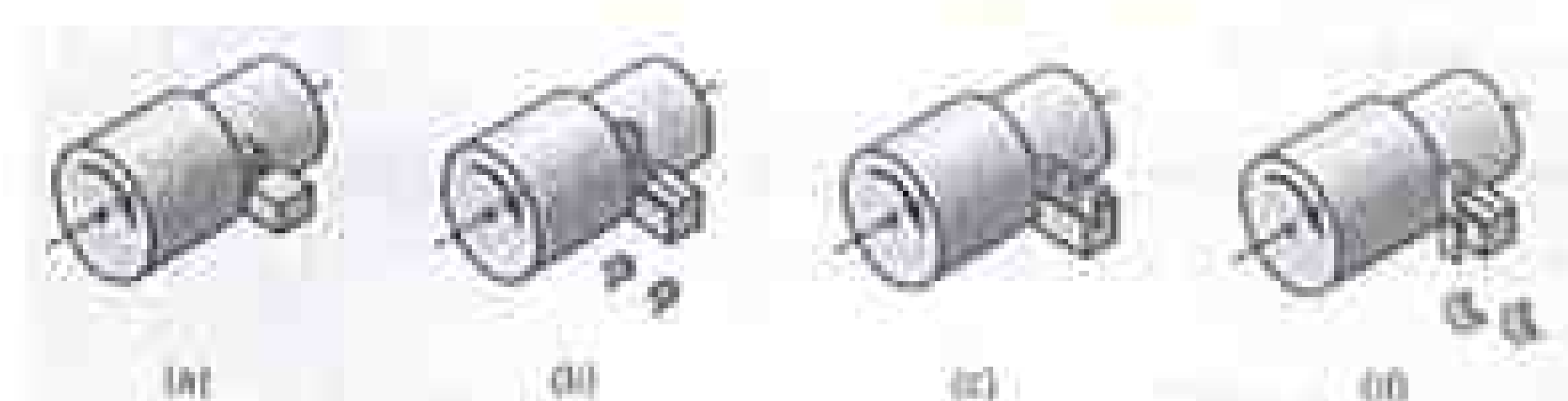
FIGURE 21.8 Chips produced in turning: (a) rightly curled chip; (b) chip hits workpiece and breaks off; (c) continuous chip moving radially away from workpiece; and (d) chip hits tool shank and breaks off.
