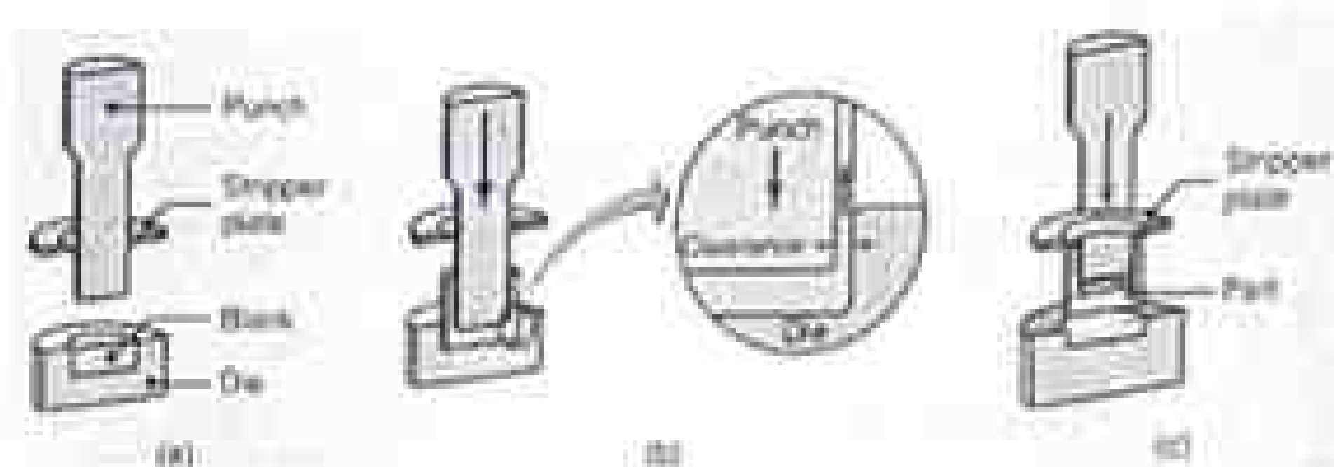
FIGURE 15.14 Schematic illustration of the impact-extrusion process; the extruded parts are stripped by using a stripper plate.
